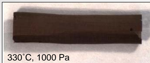
SM-10 – Some Distortion and Cracking
