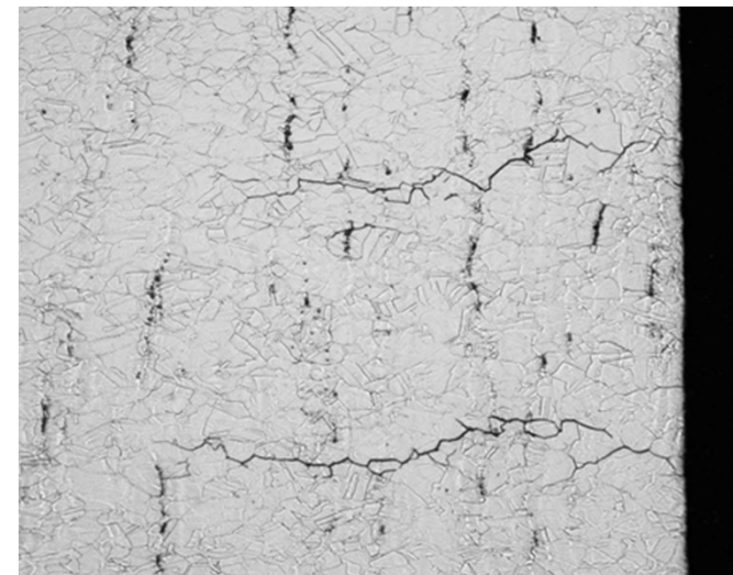
Intergranular Cracking -characteristic of hydrogen embrittlement
